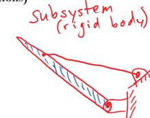
2. Draw free body diagram showing ALL the external (applied loads and supports)
