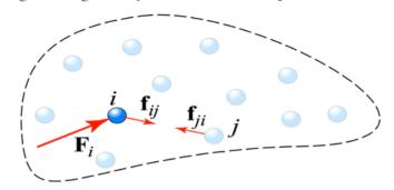
We can reduce the force and couple moment system acting on a body to an equivalent resultant force and a resultant couple moment at an arbitrary point O.
